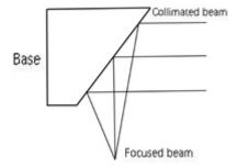
GCC-501 series OAPs adopt high-quality aluminum with a metal reflective coating on the parabolic surface. There are three types of reflection coatings: protective gold, protective silver and UV enhanced aluminum.
